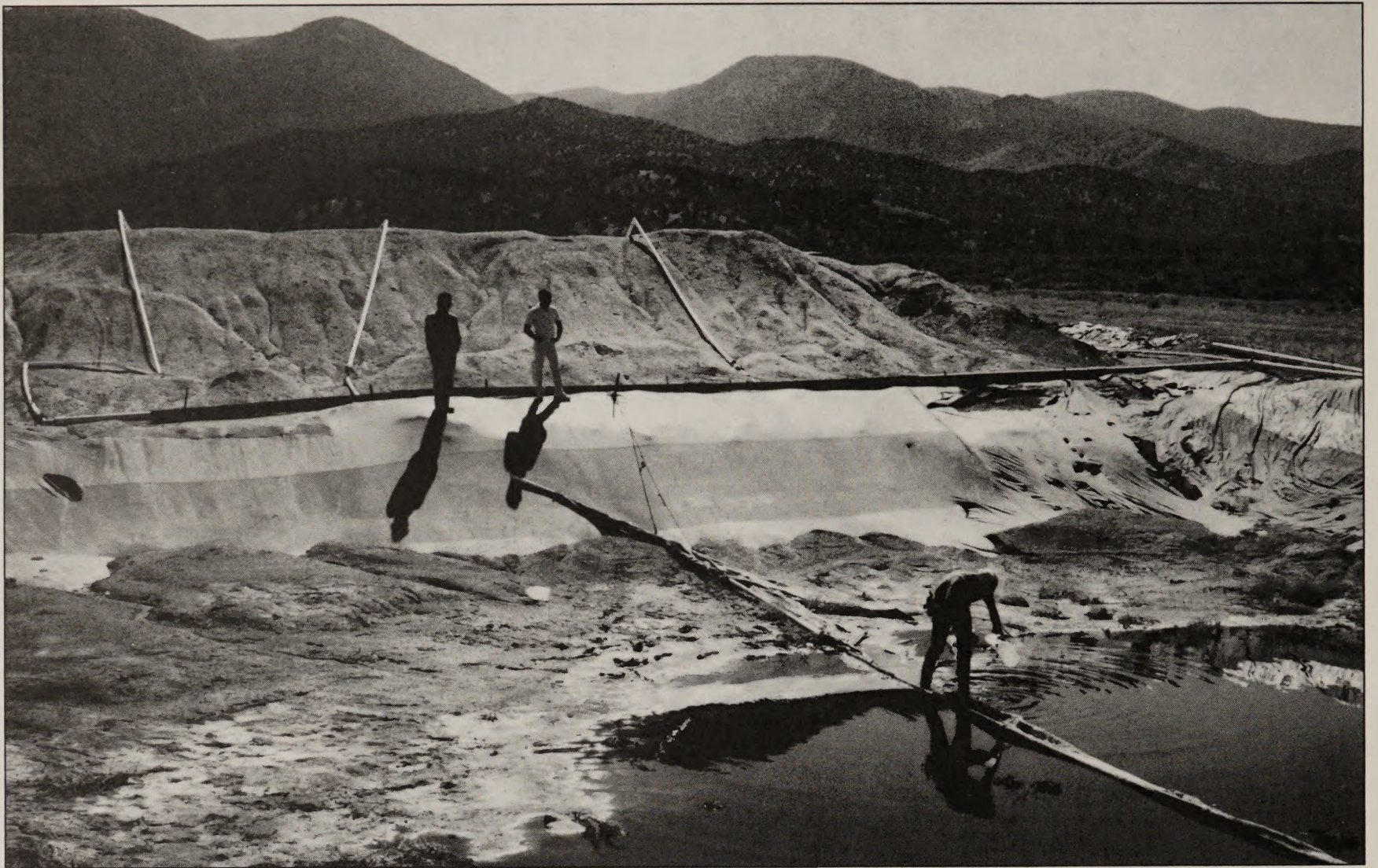
Figure 4. A representative from Barrick Mercur Mines is sampling the solution pond after hypochlorite has been added to neutralize the cyanide.
